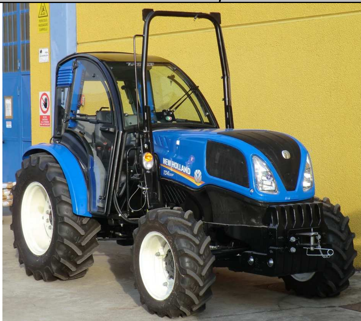
“COMPACT” Cabin NEW HOLLAND TD4.100F Back Tyres 380/70 R.24
