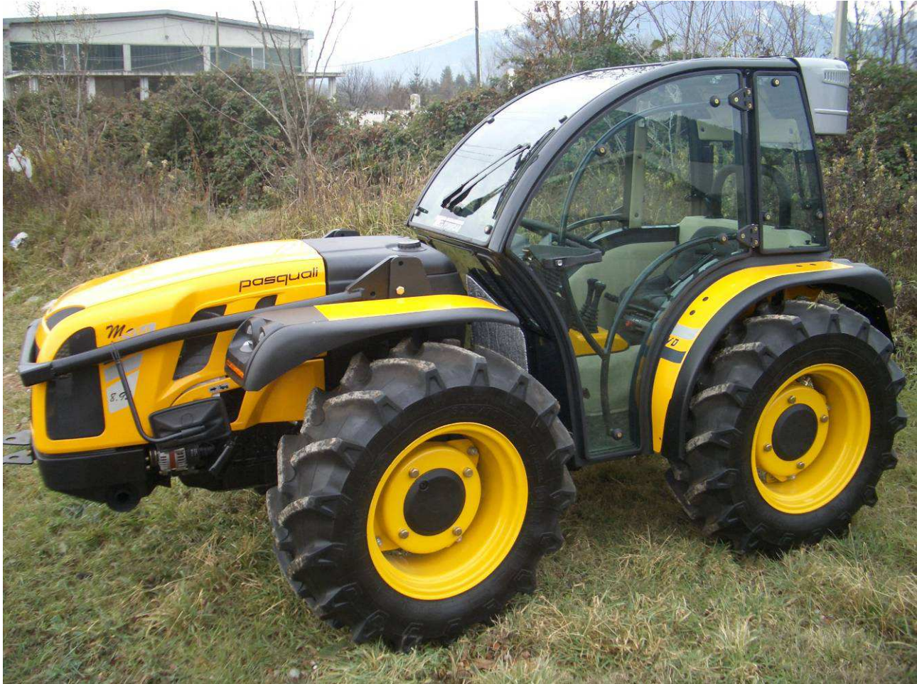
“COMPACT” Cabin PASQUALI MARS 8.95 RS Monodirectional Tractor Tyres 280/70 R.18
