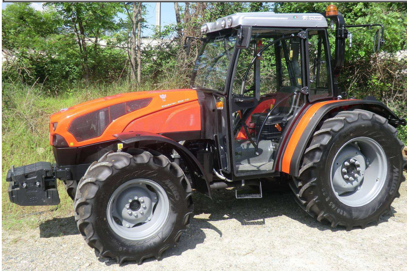
Cabina SAME EXPLORER 105 TB Stage IIIB Gomme posteriori Trattore 480/65 R.28
